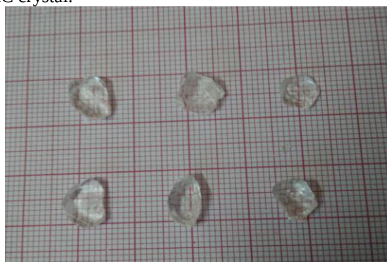
Figure 1: The grown crystal of gamma glycine using rubidium chloride as an additive (GGRC)
