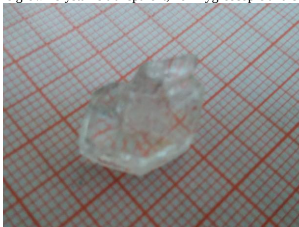
Figure 1: As-grown crystal of ammonium cadmium sulfate hydrate
