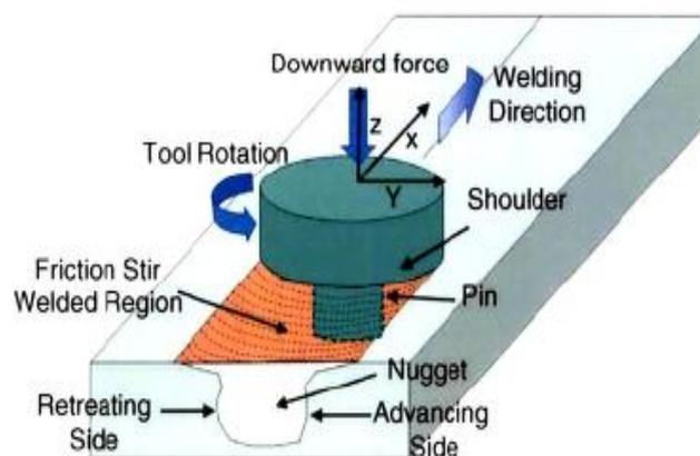
Figure 1: Schematic layout of friction stir weld Tool.
