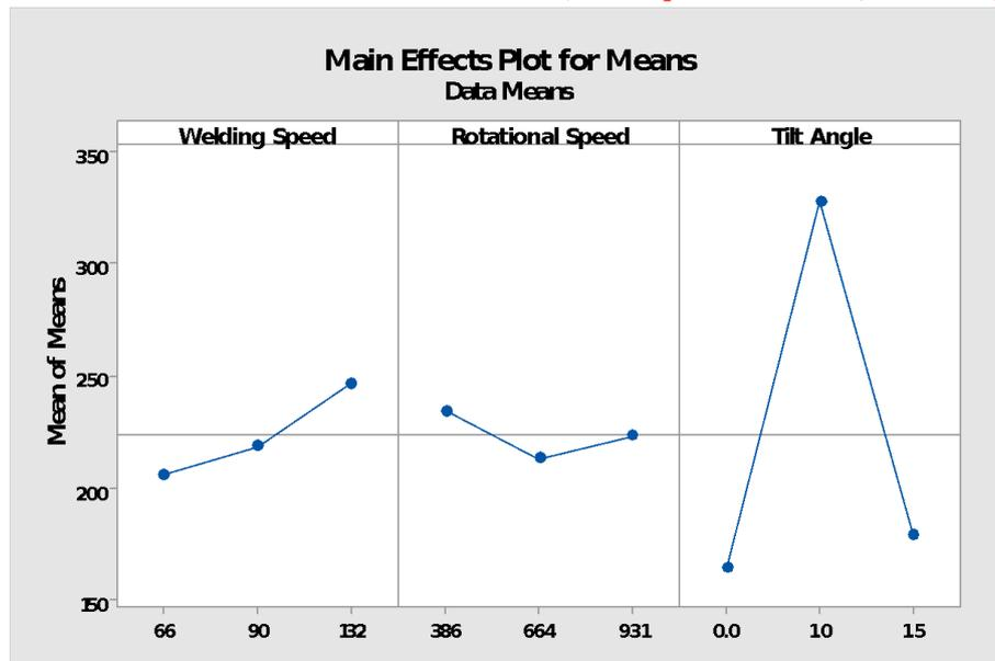
Figure 3: Main effects plot of mean data for UTS on Friction stir welding process
