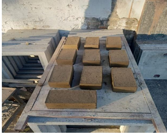
Figure 4: Initial drying process of Gaucrete bricks
