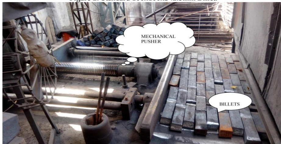
Figure 3: Billets are pushed into a reheating furnace by a mechanical pusher.
