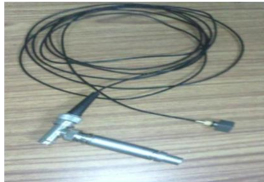
Figure 2: Accelerometer with Cable and Connector
