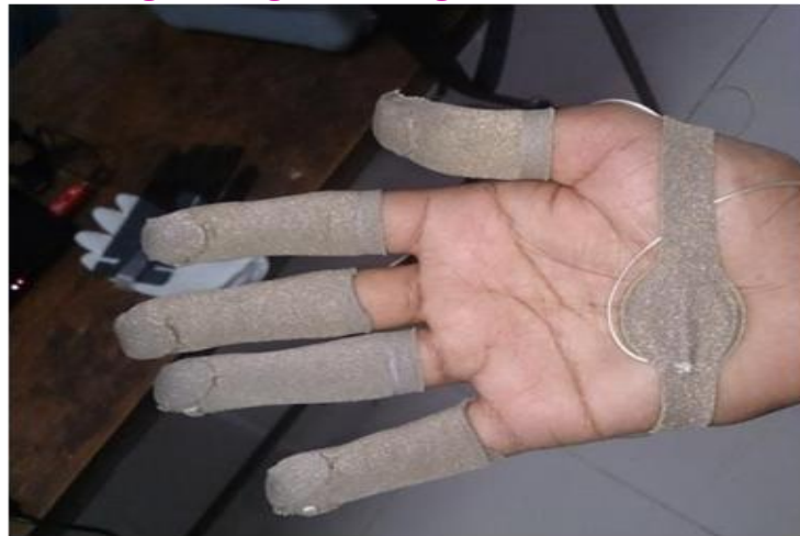
Figure 7: Sensors setting up on fingers
