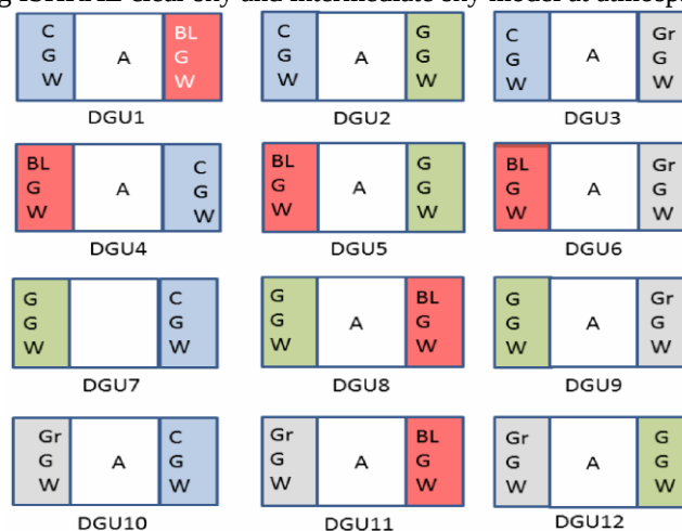
Figure 1: Double window glass units with an air gap 10mm
