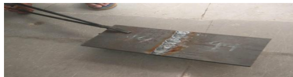
Figure 5: Butt joint of first pairs
