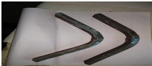
Figure 23: After bend test of first specimen
