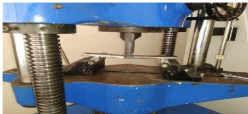
Figure 21: Specimen under bend test
