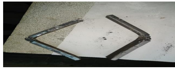
Figure 24: After bend test of second specimen
