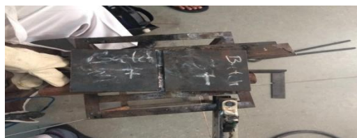
Figure 6: Welding of plates using SS as filler material
