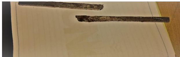
Figure 33: Specimen after tensile test
