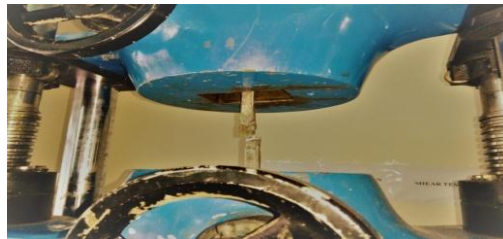
Figure 27: specimen fractured during tensile testing
