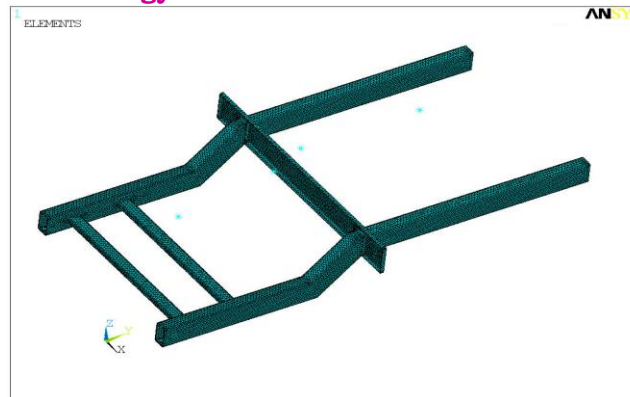
Figure 3: FE Model of 3 wheeler passenger vehicle chassis
