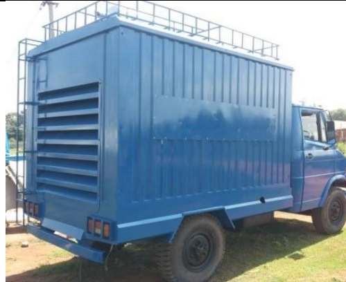
Figure 7: Acoustic Enclosure for Mobile DG Set
