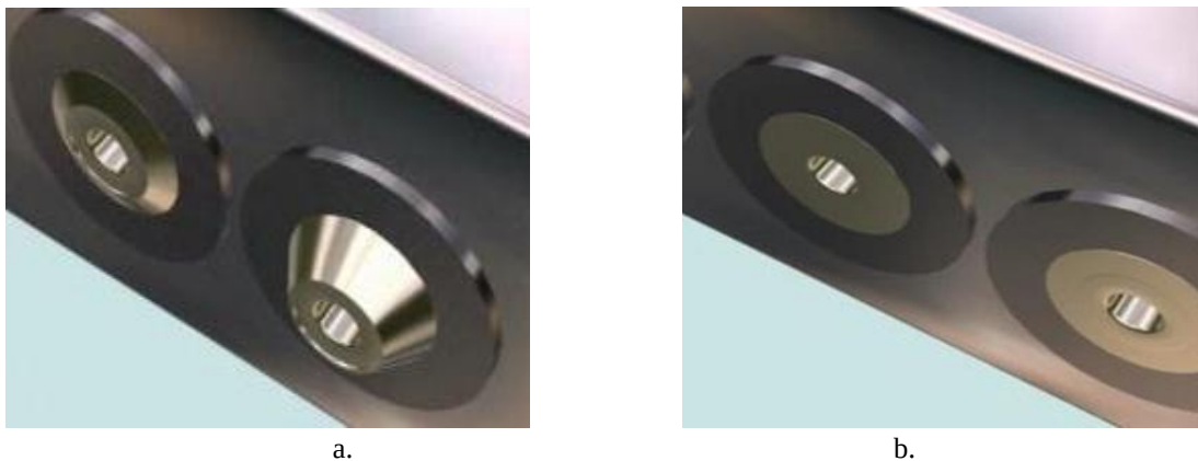
Figure 5: Die Assembly at the station 3 and 4 for a) trimming and b) forming version
