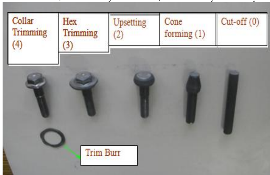
Figure 2: Stage Samples of Forging (trimming Version)
