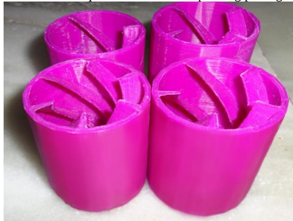
Figure 2.1: Helical guide vane swirl devices produced from 3 D printing
