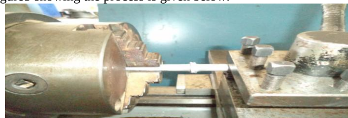
Figure 5: Both the components joined together post welding. Post processing can be done if required
