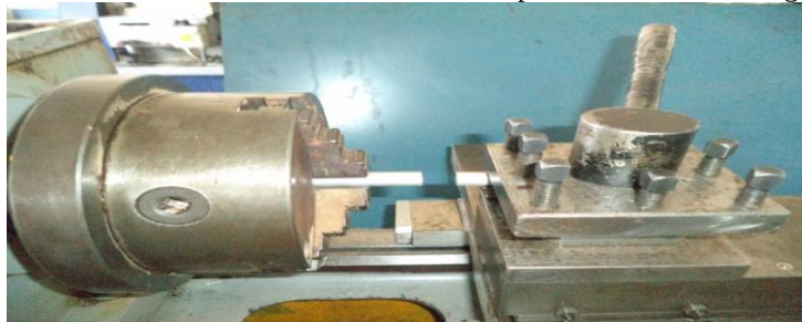
Figure 3: Two aluminum rods fixed to the lathe machine. One to spindle and another to tool post
