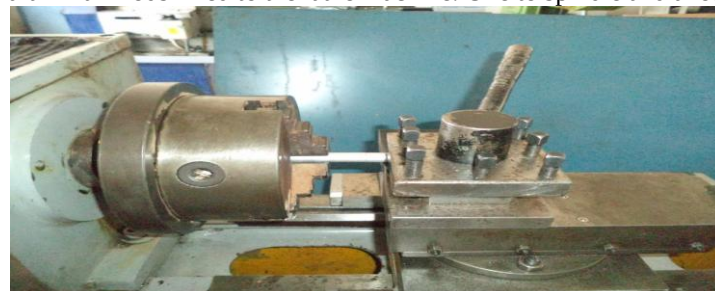
Figure 4: Axis of both the components are aligned and brought close to each other
